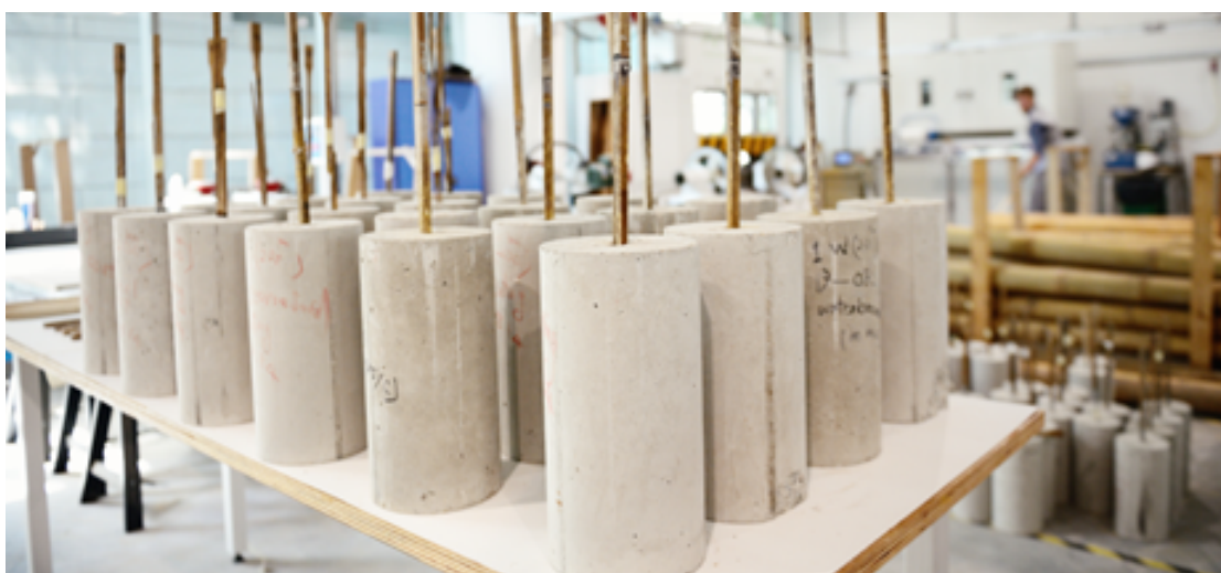
Pull-Out Test for Bamboo Composite Reinforcement at the Advanced Fibre Composite Laboratory. This work is led by Asst Prof Dirk E Hebel of the Singapore ETH Centre.
